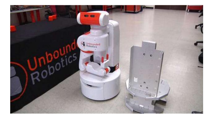
Unlike the industrial robots widely used in manufacturing today – usually large machines isolated from people for safety reasons – this robot can work alongside humans or autonomously in a workspace filled with people.
