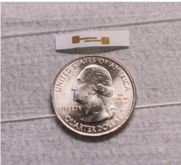
Led by Dr. Shalini Prasad, a team at the university is creating an electrochemical biosensor that continuously measures glucose in the wearer's sweat.
