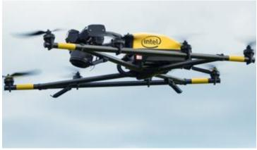
Intel's expert-level drone builds on the <u>AscTec Falcon 8</u> <u>drone</u>, a V-form octocopter that boasts high stability, precision GPS and flight control electronics and components that are redundant three times over, as well as laying claim to the best weight-to-payload ratio around (empty weight 1.1 kg, max. payload 0.8 kg). This is basically an industrial drone designed for some of the most intense field applications.
