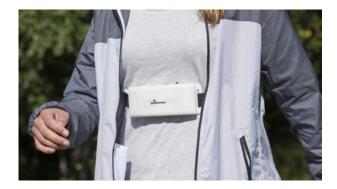
For one, the device can be worn in a low-profile way. "Guidesense functions based on radio waves, so that the signal passes through normal clothing," says VTT Senior Scientist Tero Kiuru. "This means that it can be worn discreetly under a coat, for example." That also means it's compatible with other common aids, such as using a cane, dog, or reflective vest.
