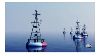
According to DARPA, the TUNA project is a selfpowering, quickly-deployable RF network that uses buoys connected by thin underwater fiber optic cables that are designed to last up to 30 days – the agency believes is enough time to bring the damaged primary network back online. The recently completed Phase 1 was intended to develop concepts and technologies in the fields of modelling and simulation, as well as at-sea testing of the buoys and cables.
