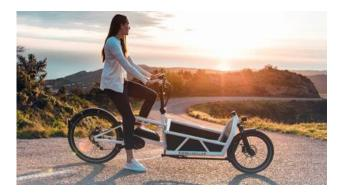
The Load has a fairly conventional chassis design. It sits the rider at the rear, and the load down low in front of them for maximum capacity and stability without obscuring the rider's line of sight. There are a number of options for the load bay, including low and high-sidewall cargo boxes, a side-by-side child seat, or a baby-seat mount. You can also add a canvas weather shield, see-through child cover, or an elastically-attached tarpaulin.
