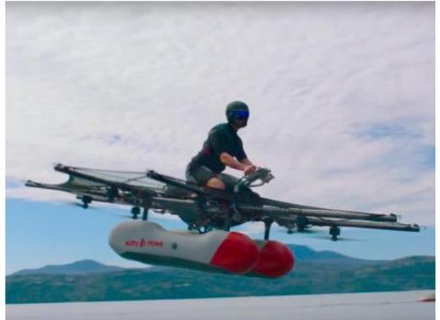
A [New York Times profile of the Flyer](#) describes it as "something Luke Skywalker would have built out of spare parts." The vehicle weighs about 100 kilograms and, according to Morrissey, can travel up to 25 mph. She likened the Flyer to "a toy helicopter."
