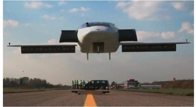
Lilium's zero-emission prototype aircraft seats two people and is powered by electric motors. It takes off vertically like a helicopter, using its vertical take-off and landing (VTOL) system, and flies using the lift from its engines.
